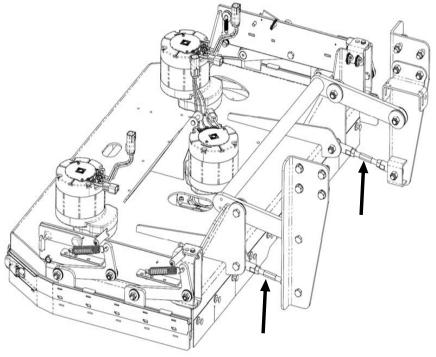
Fig. 1: Leveling Rods
