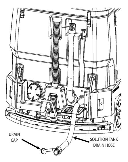
Fig. 1: Draining the Solution Tank
