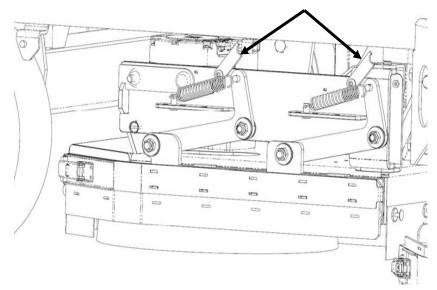
Fig. 1: Shows squeege assembly retaining arms
