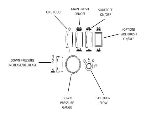
Fig. 1: Control Settings, before "One-Touch" selection
