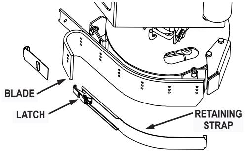
Fig. 3: Retaining Strap & Blade
