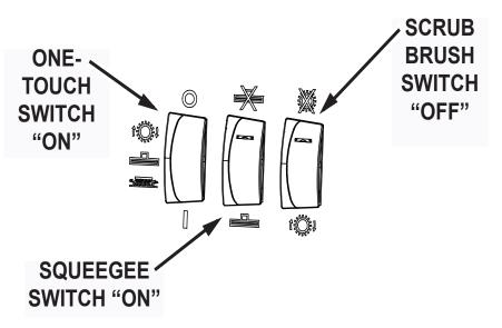
Fig. 1: Control Settings for Water Pick-up Mode
