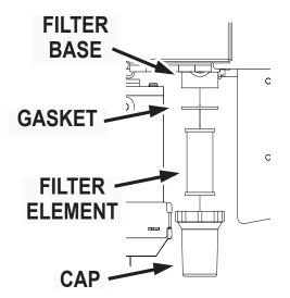
Fig. 2: Water Solution Filter with Exploded view
