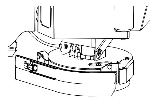
Fig. 1: Replacing the Side Scrub Brush
