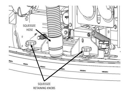
Fig. 1: Turning/Replacing the Rear Squeegee Blades
